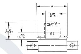
Note: Fuses with the El option are designed to work with the AOS-S or AOS-Q add-on switch, which is ordered separately. See page J6 for details.
