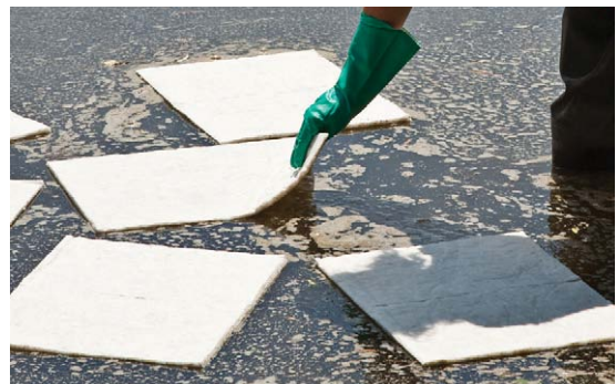
Clean up oil and petroleum-based spills on land or water with specialized sorbents that don't absorb water.
