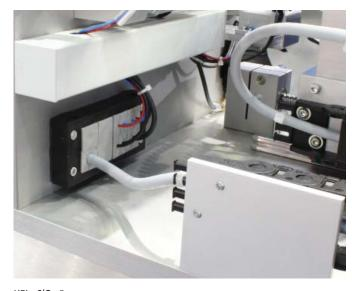
**KEL 16|8 -** Page 10 Routing of several pre-terminated lines into the electrical enclosure of a tension measuring machine.
