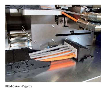
Used in combination with cable carriers to provide strain relief and compact, high density cable entry into control enclosures.
