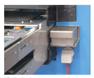
**KVT 50-W90** - Page 46 Low profile 90 degree routing of a terminated cable from a control panel into the machine
