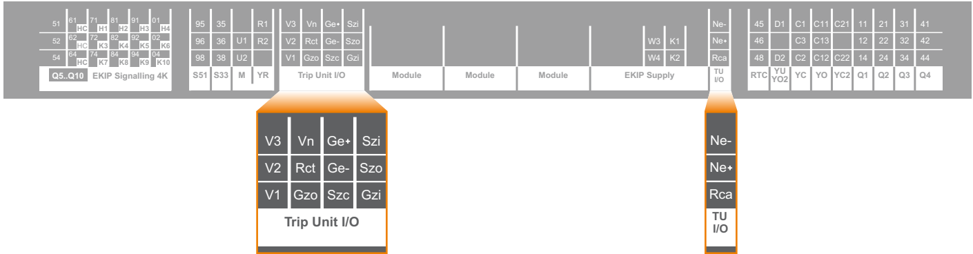
24) Rc residual current protection sensor input (ANSI 64 & 50NTD) 24a) Rc differential ground fault protection (ANSI 87N)
