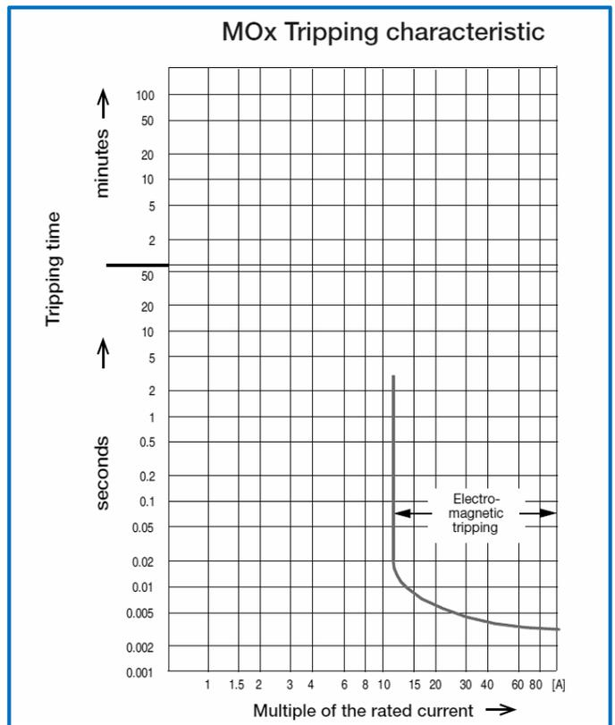
The tripping characteristics for manual motor starters can be accessed in the Download Center (<http://www.abb.com/abblibrary/downloadcenter>).
