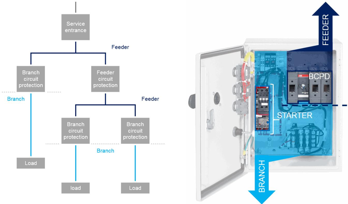
Manual motor starters, when tested as Combination Motor Controllers Types E or F, are suitable for branch circuit protection. However, these devices cannot be used for providing protection of feeder circuits. Feeder circuit protection is typically provided using either fuses, UL 489 / CSA C22.2 No.5 molded case or UL 1066 / CSA C22.2 No.31 power circuit breakers.
