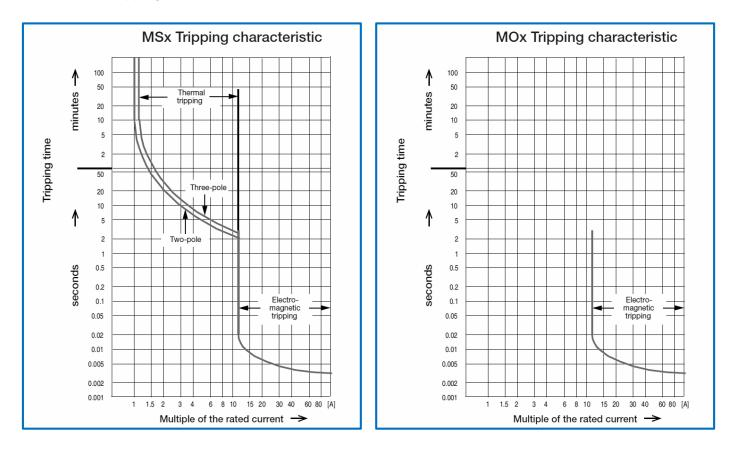
The tripping characteristics for manual motor starters can be accessed in the Download Center (http://www.abb.com/abblibrary/downloadcenter).
