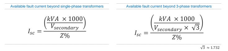
The available fault current directly at a transformer's secondary terminals  $I_{sc}$  can be calculated from the transformer full-load current *kVA*, the secondary voltage line-to-line  $V_{secondary}$  and the transformer impedance *Z*%. For transformers with an unmarked impedance, this can be assumed to be 2.1% (0.021  $\Omega$ ).
