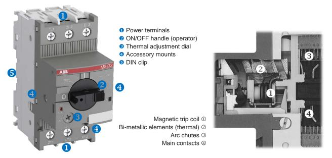
Control and disconnect functionality is realized through the rotary-style knob on the device face. Protective functionality is realized through the internal releases (tripping elements), which provide:
