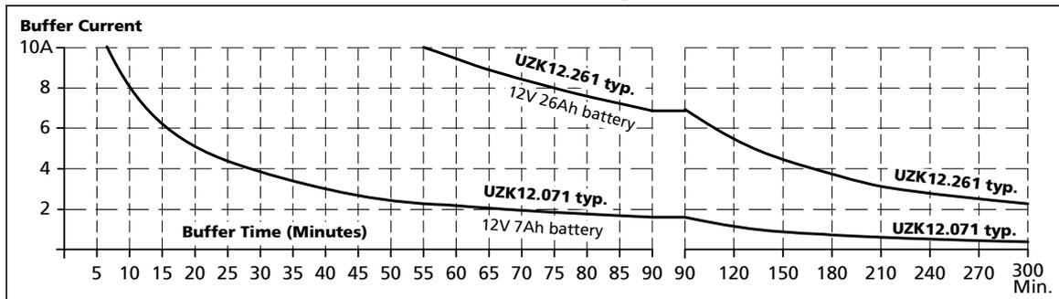
The battery capacity is usually specified in amp-hours (Ah) for a 20h discharging event. The battery discharge is non-linear (due to the battery chemistry). The higher the discharging current, the lower the appropriate battery capacity. The magnitude of the reduction depends on the discharging current as well as on the type of battery. High current battery types can have up to 50% longer buffer times compared to regular batteries when batteries will be discharged in less than 1 hour.
