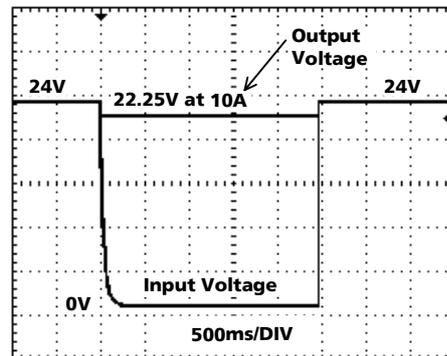
Fig. 7-3 Available output current in buffer mode
