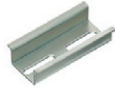
TS 35/15 mm according to EN 50022 (s = 1.5 mm)
