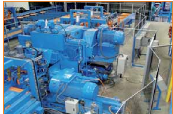
Quick-Guard E with few components and easy to angle at up to 20°.
