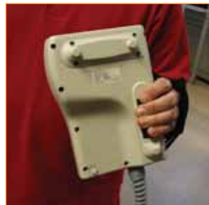
Panel assembly of JSHD4H2 on a programming unit for robots.
