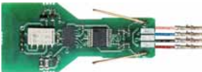
Anti-tamper PCB – 2TLA020005R0900
