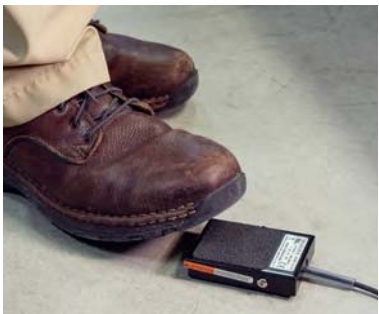
Use the foot pedal to trigger sleeve removal from liner
