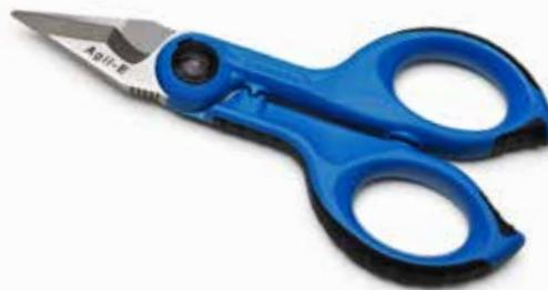
Only 0.2 lbs weight, the tapered blades and streamlined handles encourage agility and speed of operation. Handles have an integrated crimping system for end sleeves. **Cutting of flexible conductors up to 1/0 AWG**
