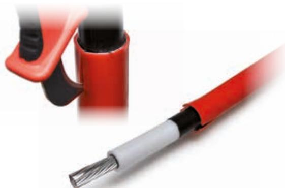
Insulated knife, with curved blade and protective cover. Suitable for insulation and screen removal, equipped with blade guide to avoid damage to strands. Handle is made of a bi-component plastic material.
