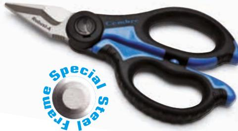
Professional scissors with **Special Steel frame**, high hardness blades (58 HRC) and anti slide serrations. The moulded plastic handles combine a rigid structure with a softer material for finger comfort. **Cutting of flexible conductors up to 1/0 AWG**
