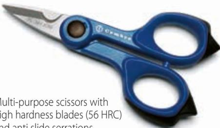
Multi-purpose scissors with high hardness blades (56 HRC) and anti slide serrations. The moulded plastic handles combine a rigid structure with a softer material for finger comfort. **Cutting of flexible conductors up to 2 AWG**
