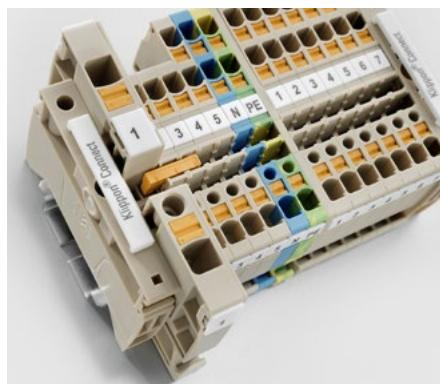
The ALO 6 supply terminal can be used for supplying current up to a conductor cross-section of 6 mm<sup>2</sup>. Standard cross-connections then distribute the current to any number of terminals with a smaller cross-sectional area.
